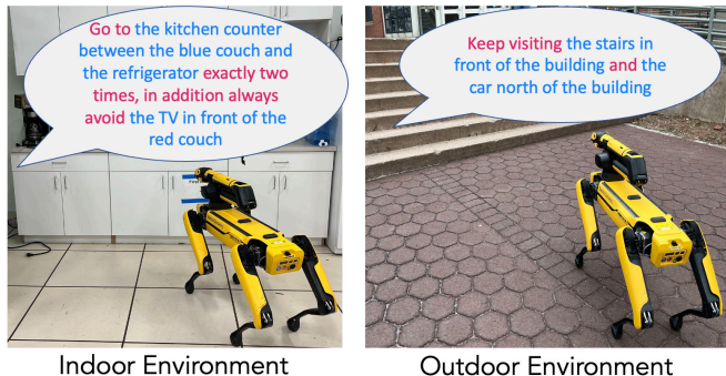
Fig. 1: Our system Lang2LTL-2 grounds spatiotemporal navigation commands in indoor and outdoor environments. The spatial and temporal elements of the example commands are highlighted in blue and red, respectively.
